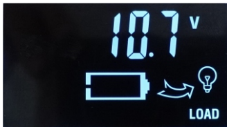
8: Discharge cut-off voltage setting
