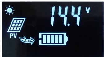
6. Floating charge voltage setting
